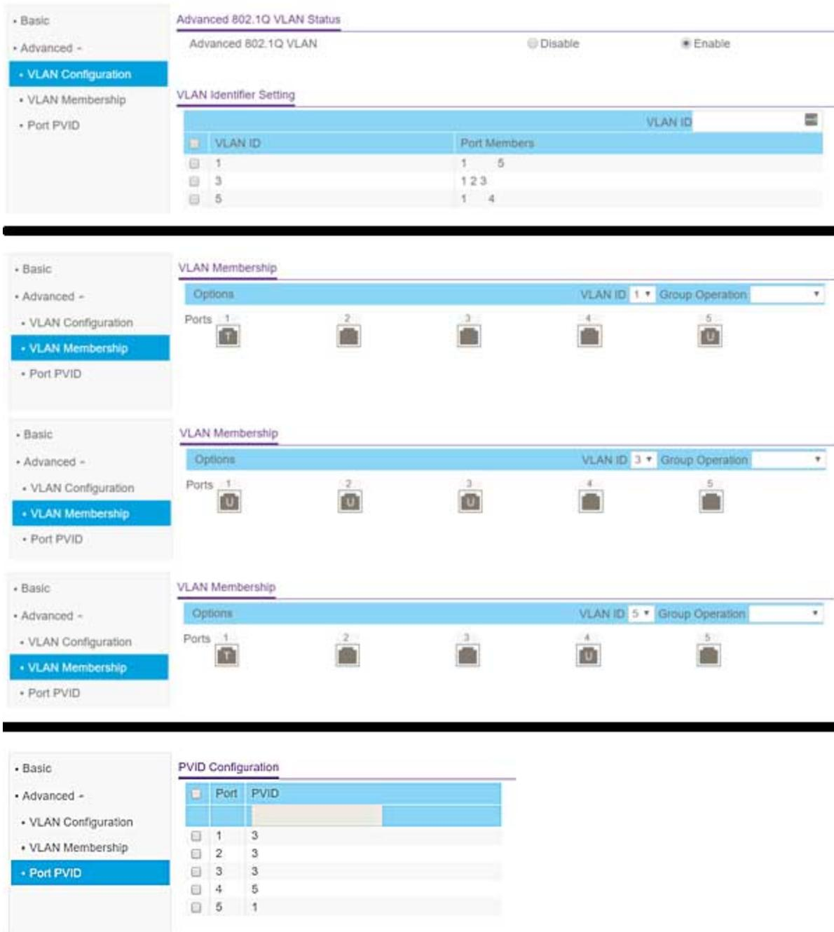
Figure 3 - 802.1Q Advanced VLAN configuration inside the GS105 switch.
