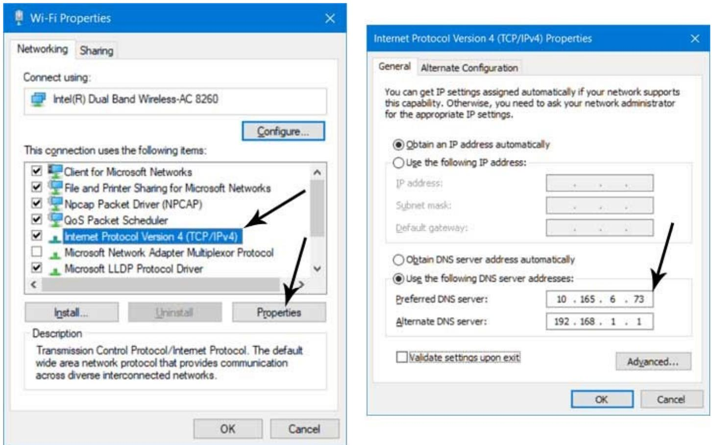
Figure 8 - Windows IPv4 properties for the Wi-Fi network adapter. Do the same for all network adapters needing DNS for your mesh node.
