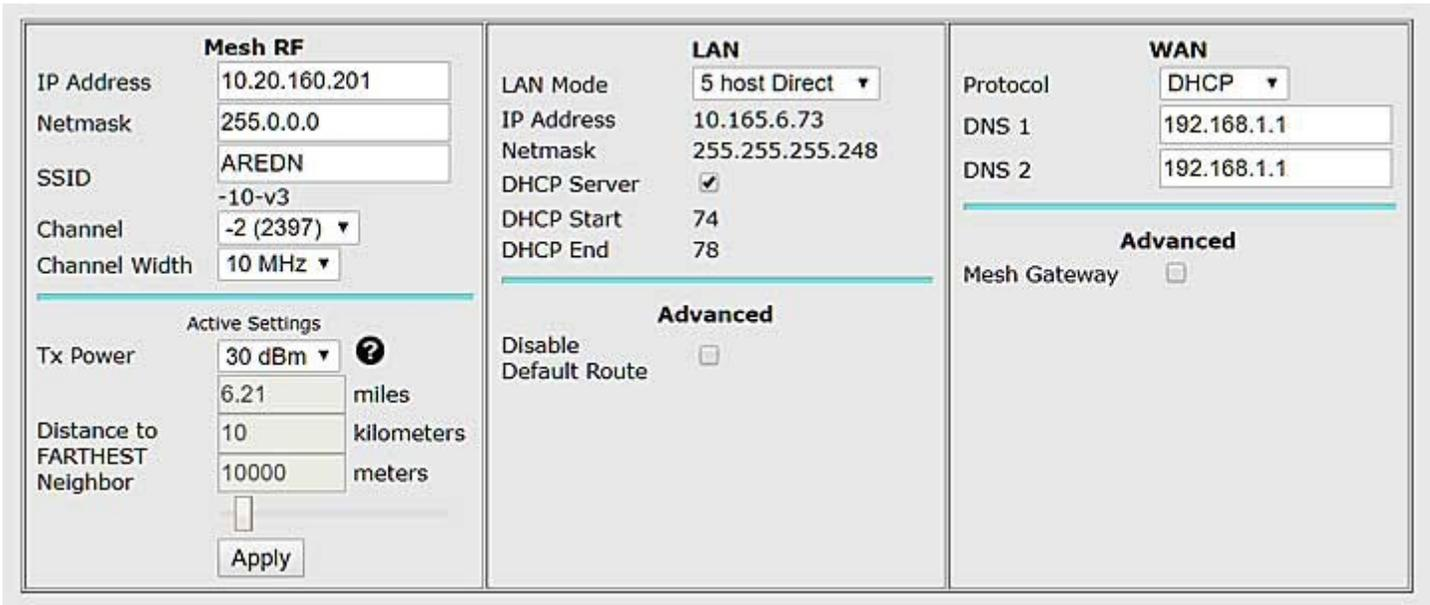
Figure 1 - The AREDN mesh node Basic settings screen
